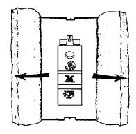
4. Lower Element: Lift out the tab as shown to unclip the terminal cover from the thermostat. The terminal cover can be removed from the thermostat.
